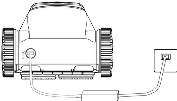
1. Plug the adapter into power supply and make sure that indicator light is being red.
